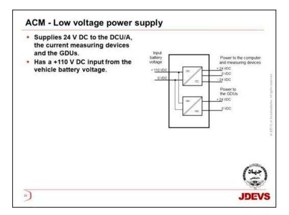
In the MCM there is a low voltage power supply to supply the MCM computer and the current measuring devices with 24 V DC. The power supply also supplies the Voltage Measuring Board (VMB) and the GDUs with +24 V DC.
