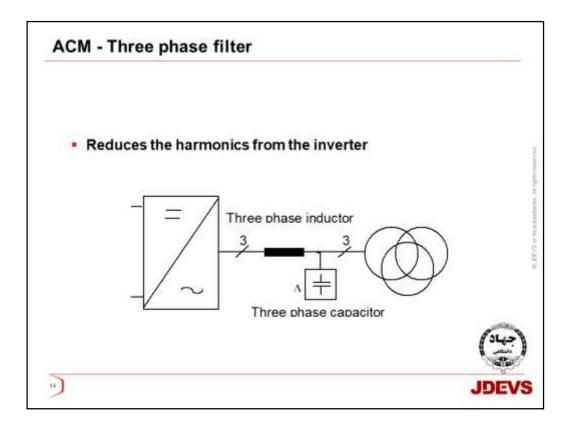
At the output of the IGBT inverter there is a **three phase filter** to reduce the harmonics generated by the inverter. The filter consists of a three phase inductor and a three phase capacitor.
