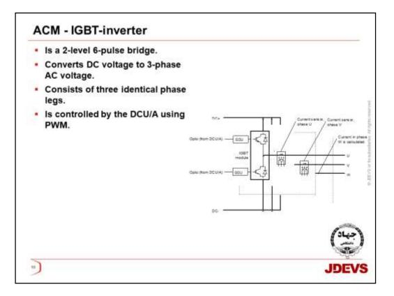
The inverter is a 2-level 6-pulse bridge which converts DC voltage to 3phase AC voltage. It consists of three identical phase legs. The switching elements are high voltage IGBTs. The inverter is controlled by the DCU/A using a Space Vector Modulation (SVM) technique which is a well known PWM (Pulse Width Modulation) algorithm.
