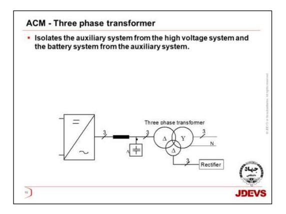
The transformer has three windings, one primary, one secondary for the three phase load and one secondary for the battery rectifier. The transformer isolates the auxiliary system from the high voltage system and the battery system from the auxiliary system. The voltage ratio of the transformer is 270/400/92 V at rated load.????
