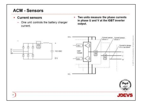
There are three current sensors in the ACM. Two sensors measure the phase currents on the output side of the inverter. One sensor measures the battery charger current on the output side of the battery charger.
