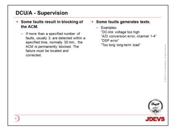
The ACC/I supervises and protects the functions and equipment in the ACM. Some faults result in blocking of the ACM. If more than a specified number of faults, normally three, are detected within a specified time, normally 30 minutes, the ACM is permanently blocked. In such this cases the failure must be located and corrected.
