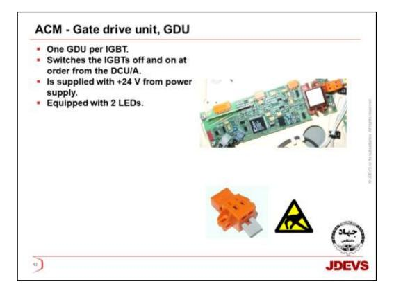
The **gate drive unit** switches the IGBTs off and on at order from the DCU/A. The gate drive units can also detect phase short circuits. There are two gate drive units per phase leg, one for each IGBT.
