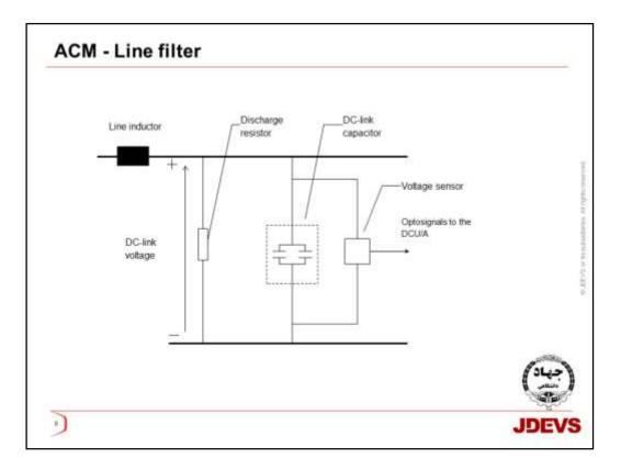
The line filter capacitor and the line filter inductor forms the line filter which filter and stabilise the DC-link voltage and is sized with sufficient capacitance to keep the voltage ripple in DC-link within permitted limits and enable accurate converter control. Link filter featuring line filter capacitor, line filter inductor, discharge resistor and a voltage sensor. In the other direction, harmonics generated by the IGBT inverter are prevented from reaching the line.
