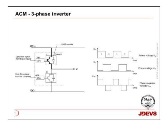
**Phase Commutation** When the upper IGBT in phase U (1) is switched ON and the lower IGBT (2) is switched OFF, the voltage output in phase U is equ-al to the DC-link voltage (DC+). When the U phase output is to be set low, an OFF order is being sent to the upper IGBT (1) and an ON order is sent to the lower (2). The phase current will be going through the free wheeling diode of the lower IGBT-module (2). The output voltage of phase U is now 0 V (DC-).
