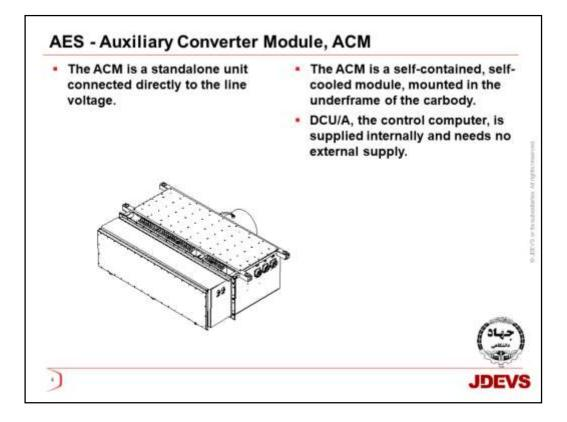
The ACM is a standalone unit connected directly to the DC-line via a main circuit breaker, a line inductor, a charging circuit and a line fuse. The ACM includes all the necessary control electronics. The control electronics are supplied from the battery system via the power supply.
