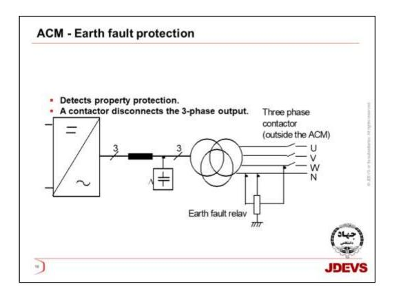
The earth fault protection consists of a resistance measuring relay connected to the neutralzero on the three phase system. The neutral, in the 3-phase system, is high ohmic connected to the earth. The relay is supplied from the phase voltage on the secondary side on the transformer.
