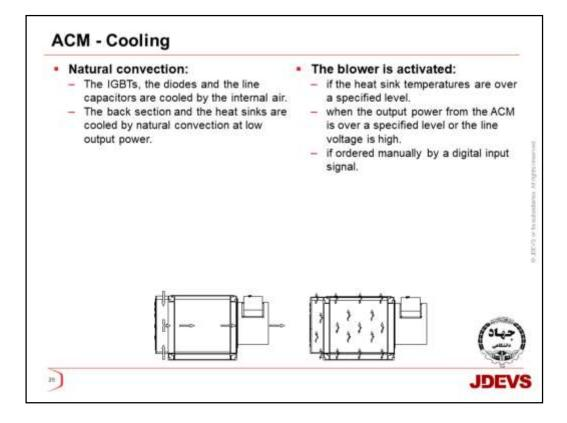
**Cooling** The ACM is designed to be cooled by natural convection at low output power. The IGBTs and the diodes are mounted on the heat sinks and the line capacitors are mounted inside the front section and cooled by the internal air.
