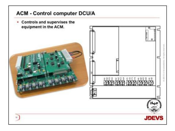
The control computer, DCU/A, in the ACM is a distributed control computer. The objective with the DCU/A distributed control is to control and supervise the equipment in the ACM e.g. the converter, the voltage and current measurement, heatsink temperatures, fan contactor etc.
