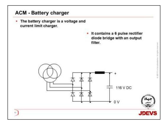
The **battery charger** is a 6 pulse rectifier diode bridge with an output filter. The secondary winding of the transformer supplies the rectifier which connects to the output filter.
