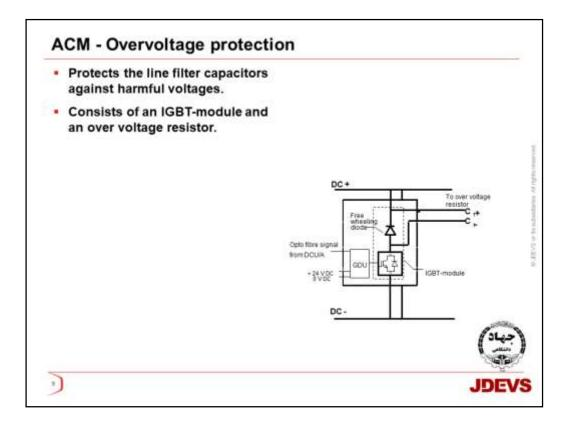
If the LFC voltage for some reason exceeds a specified level the **overvoltage protection** is activated. It consists of an overvoltage resistor in series with an IGBT. The IGBT-module consists two free-wheeling diodes, one for the IGBT and one for the resistor, which is neccessary due to their internal inductance.
